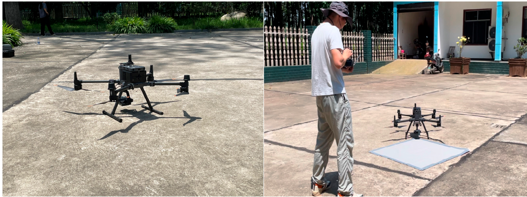
Figure 2. The DJI 350M UAV with 300TC hyperspectral camera.
