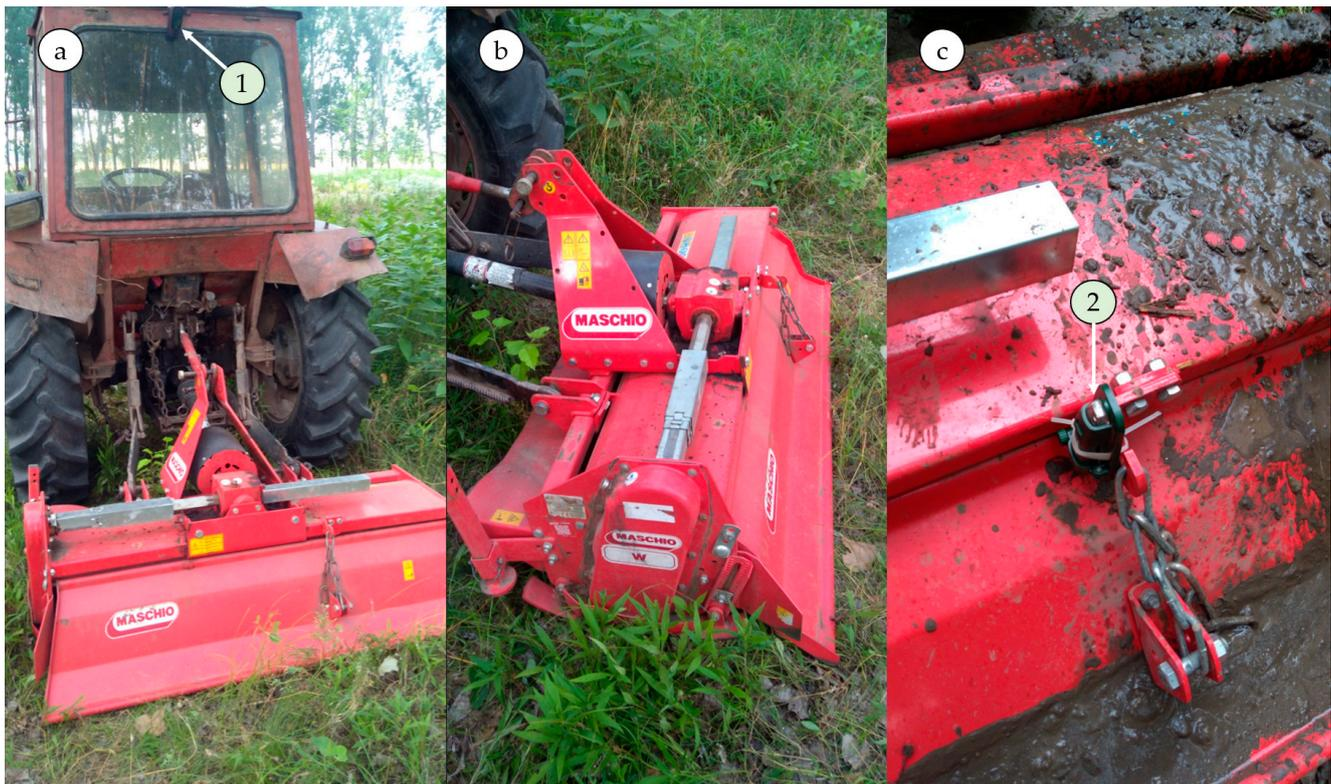
**Figure 2.** Configuration of the equipment taken into study: (a) the farm tractor equipped with the rotary tiller showing the location of the handheld GNSS receiver (1); (b) the rotary tiller observed in the study, (c) placement of the triaxial accelerometer (2) on the rotary tiller.
