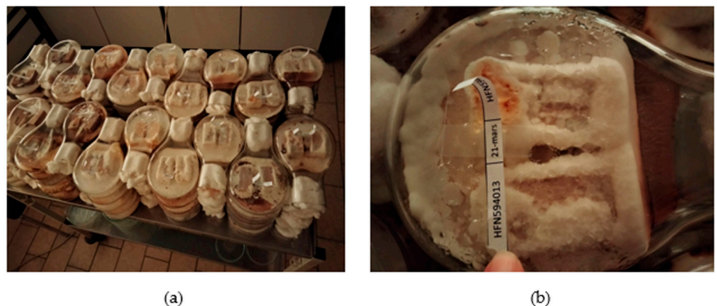
Figure 5. (a) Experiment in Kolle flasks to evaluate the wood decaying capacity of two isolates of F. fomentarius s.s. and two isolates of F. inzengae ; (b) wood specimen covered with mycelium after 16 weeks of incubation.
