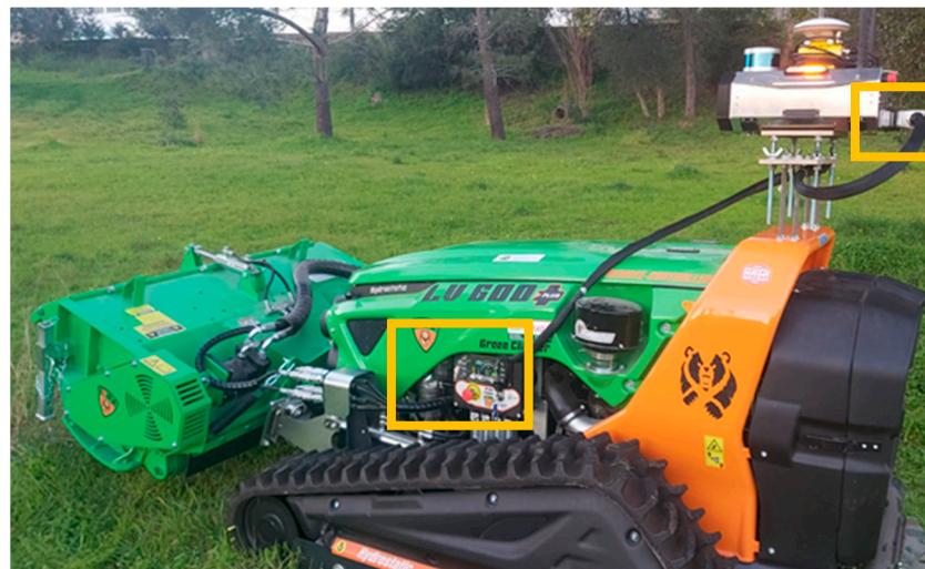
Figure 17. Connection of the sensor system into the forestry machine.
