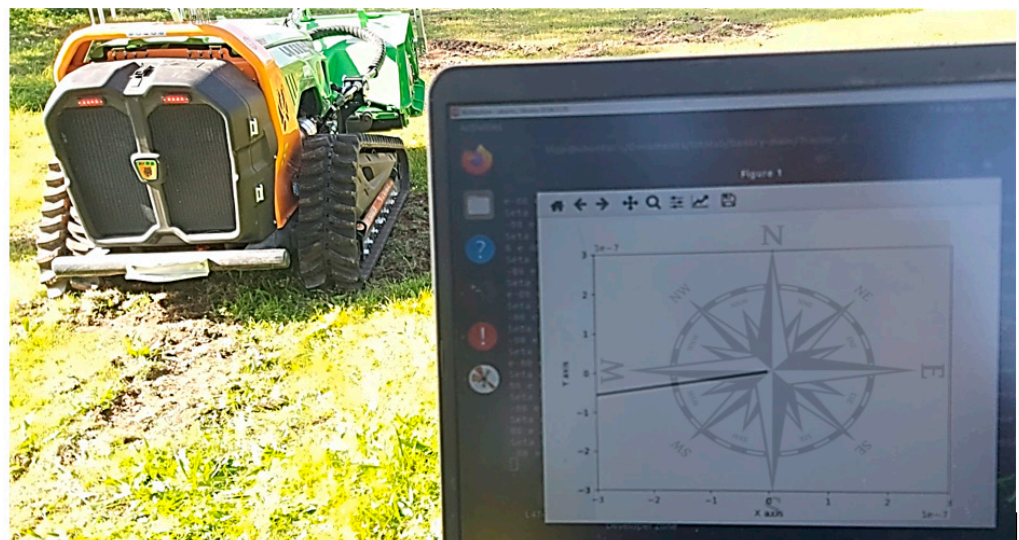
Figure 23. Experimental test for machine orientation.
