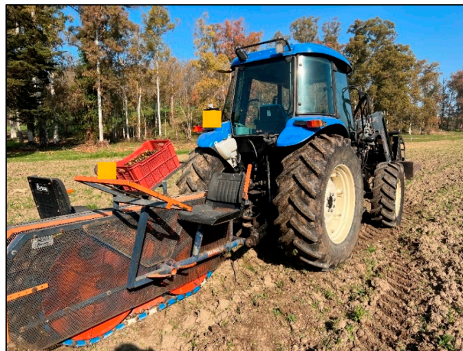
Figure 2. New Holland TD5050 crawler Rotor planter in experimental farm “Ovile” in Rome.
