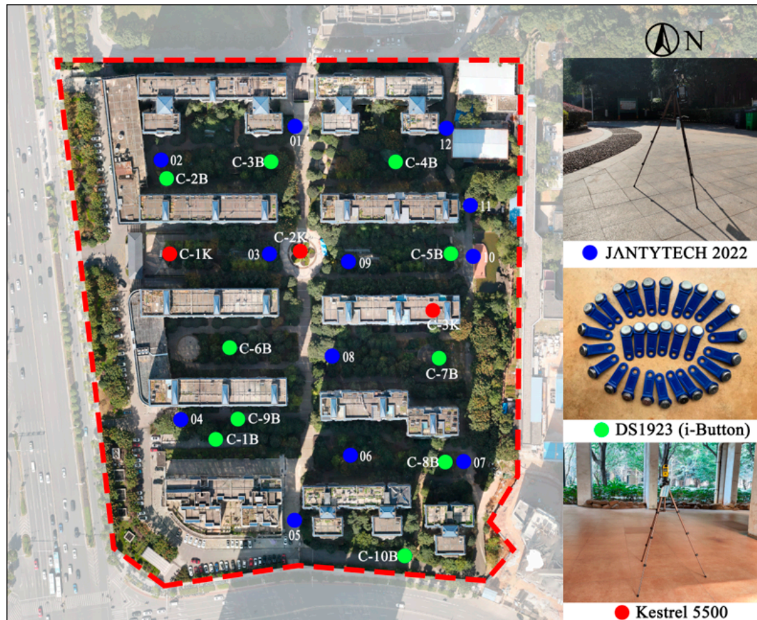
Figure 4. Layout of survey points and related instrumentation in the study area.
