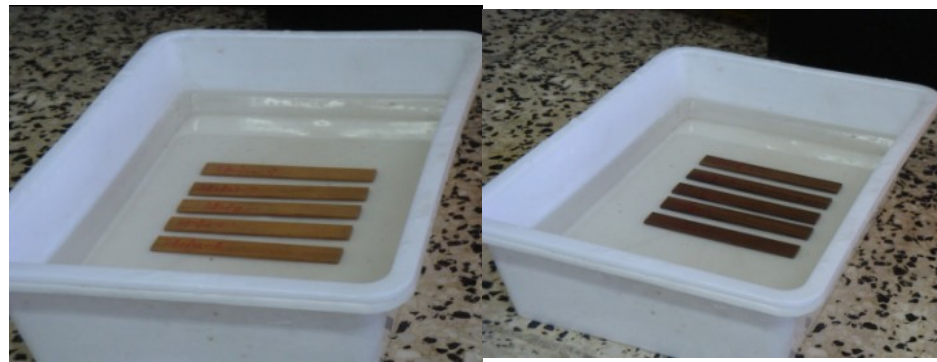
Figure 2. Water-saturated wood specimens ((left): white birch wood; (right): ash wood).
