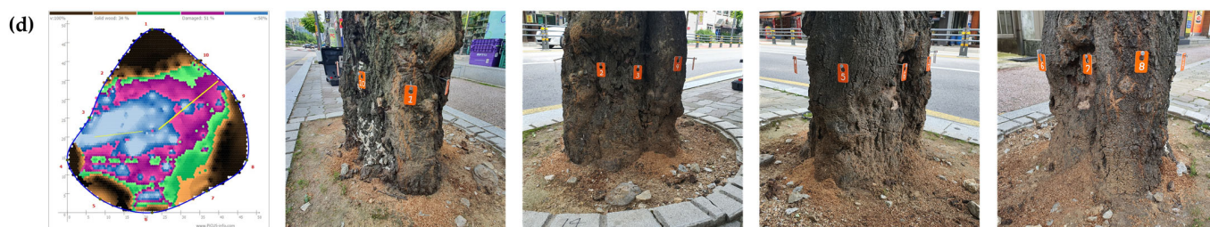
Figure A4. Representative examples of tomography of measured Quercus palustris tree (left panel) with visual images from four directions (right 4 panels): (a) non-infested tree; (b) weakly infested and 4% in injury rates in tomogram; (c) moderately infested and 25% in injury rate in tomogram; and (d) severely infested and 66% in injury rate in tomogram. The red numbers in left panels indicate the positions of the sensors. Different colors indicate wood decay severities: black and brown indicate solid wood (non-damaged areas); green is assessed in relation to the overall damage; and violet and blue indicate damaged areas (hollowed or decayed areas).
