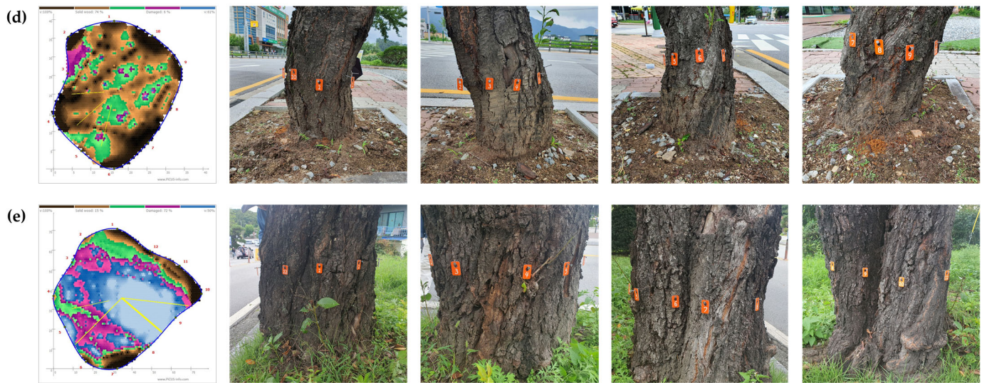
Figure A3. Representative examples of tomography of measured Prunus × yedoensis tree (left panel) with visual images from four directions (right 4 panels): (a) non-infested tree; (b) weakly infested but 0% in injury rates in tomogram; (c) moderately infested and 19% in injury rate in tomogram; (d) severely infested and 26% in injury rate in tomogram; (e) severely infested in the past and 85% in injury rate in tomogram. The red numbers in left panels indicate the positions of the sensors. Different colors indicate wood decay severities: black and brown indicate solid wood (non-damaged areas); green is assessed in relation to the overall damage; and violet and blue indicate damaged areas (hollowed or decayed areas).
