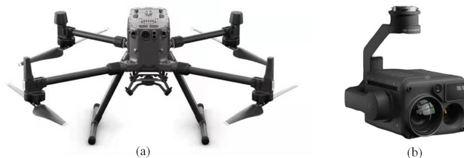
Figure 2. (a) UAV DJI-M300RTK; (b) DJI-Zenmuse H20T spectral camera.
