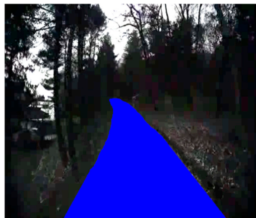
Figure 8. Forest road detection and segmentation using YOLOv8 in test image.
