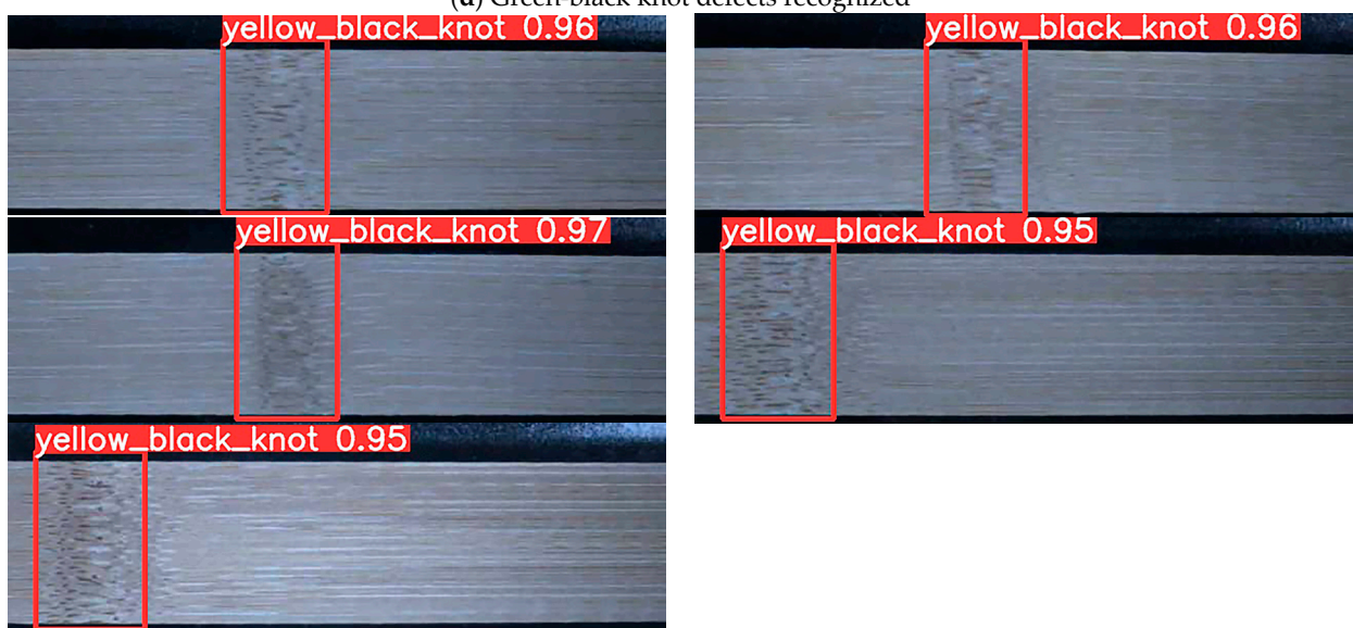
(e) Yellow-black knot defects recognized
