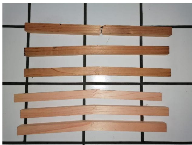
Figure 4. Bending strength tests of untreated ( bottom ) and heat-treated ( top ) Cryptomeria japonica (Thunb ex L.f.) D.Don wood.
