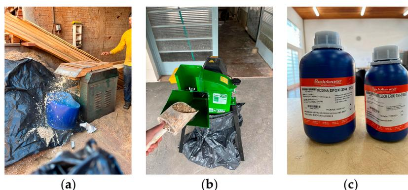
**Figure 1.** Laboratory processes: (a) pine shavings; (b) wooden particle processing using knife mill; and (c) epoxy resin and hardener.
