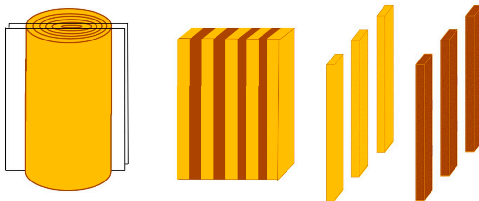
Figure 1. Scheme of preparation of the test specimens of yellow pine earlywood (EW) and latewood (LW).
