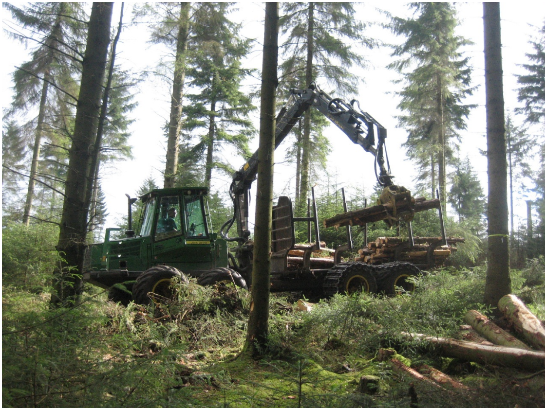
Figure 1. A forwarder extracting wood in the Clocaenog continuous cover forestry (CCF) Research Forest in northeast Wales. Recently CCF has become an accepted approach to forest management in Britain but uncertainty about its economic consequences may be a barrier to its wider use.
