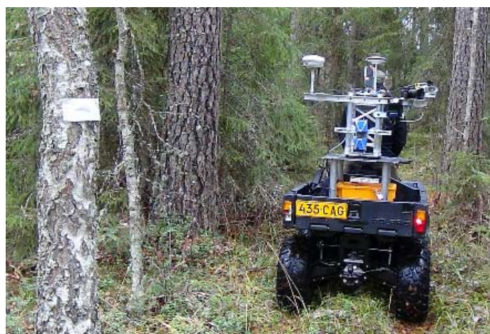
Figure 1. An ATV with global satellite navigation systems (GNSS) antennas and receivers, inertial measurement unit (IMU) and laser scanner equipment mounted on it for the purposes of the study.
