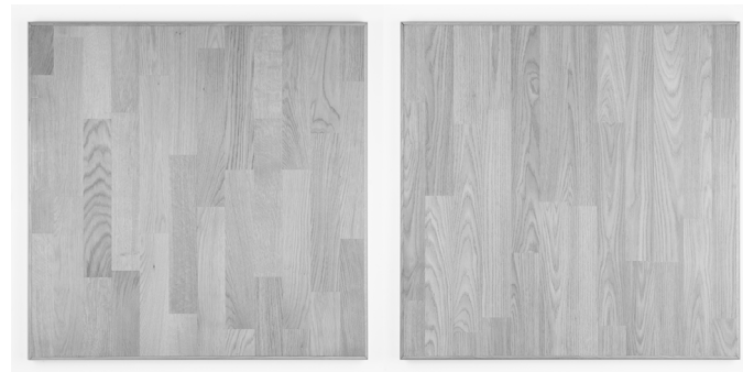
Figure 1. Framed floor pieces. (Left) oak hardwood (floor A); (right) laminate with oak optic (floor B).
