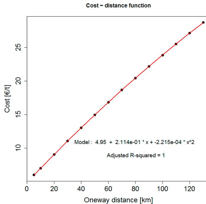
**Figure 3.** Linear model with 2nd degree polynomic function (red line) modelling the relationship between transport distance and cost per dry Mg of woody biomass. Data points are the black dots.
