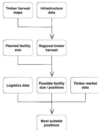
**Figure 1.** Simplified workflow of the approach showing necessary data and intermediate results for finding the most suitable facility positions.
