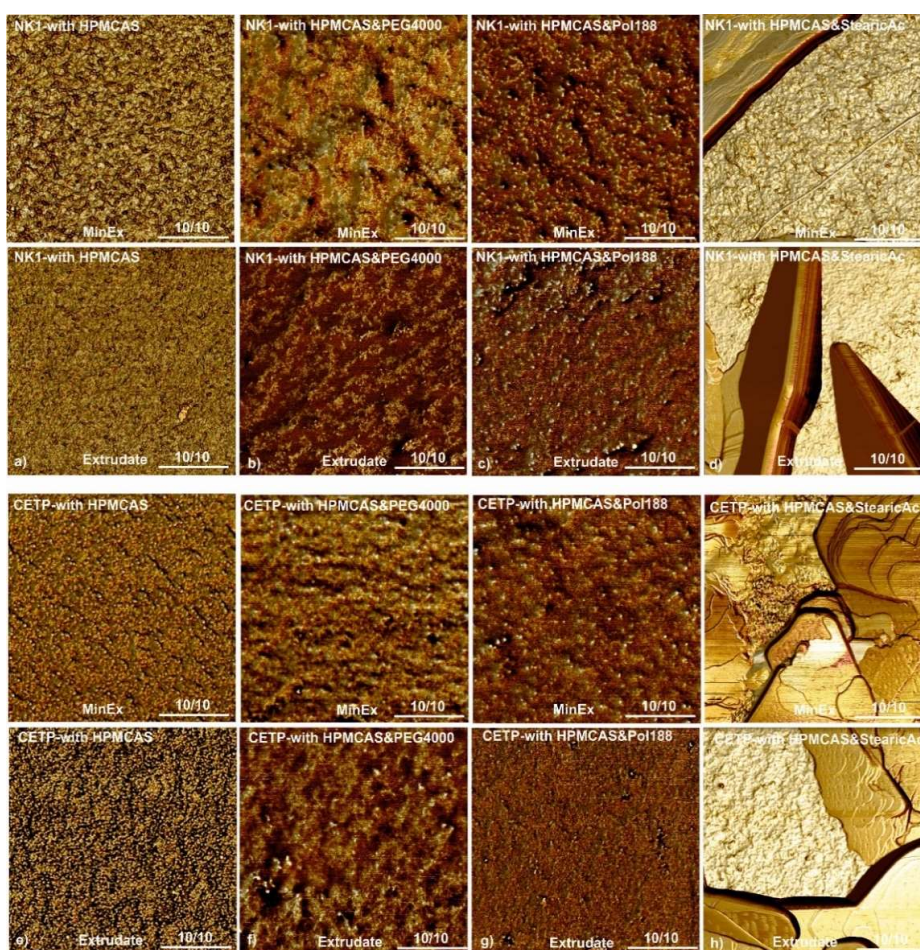
Figure 10. Phase maps recorded with tapping mode AFM on fracture surfaces of extrudates which have been exposed to temperature humidity stress storage for 2 h, T = 40\text{ }^{\circ}\text{C} and \text{RH} = 75\% , NK1 series (a–d) and CETP2 series (e–h). Row 1 shows NK1-MinEx and row 2 shows NK1-lab-scale extrudates. Row 3 shows CETP-MinEx and row 4 shows the CETP-lab-scale extrudates. Similarly composed extrudates are grouped in columns. Binary systems with HPMCAS are shown in column 1, with HPMCAS + PEG4000 in column 2, with HPMCAS + Pol188 in column 3 and with HPMCAS + SA in column 4. The scale bars in all images are identical and correspond to a lateral distance of 1\text{ }\mu\text{m} , the numeric ratio shown above indicates the overall reproducibility of the observation. A ratio of 10/10 suggests that the other 9 investigated regions which are not shown here showed comparable features.
