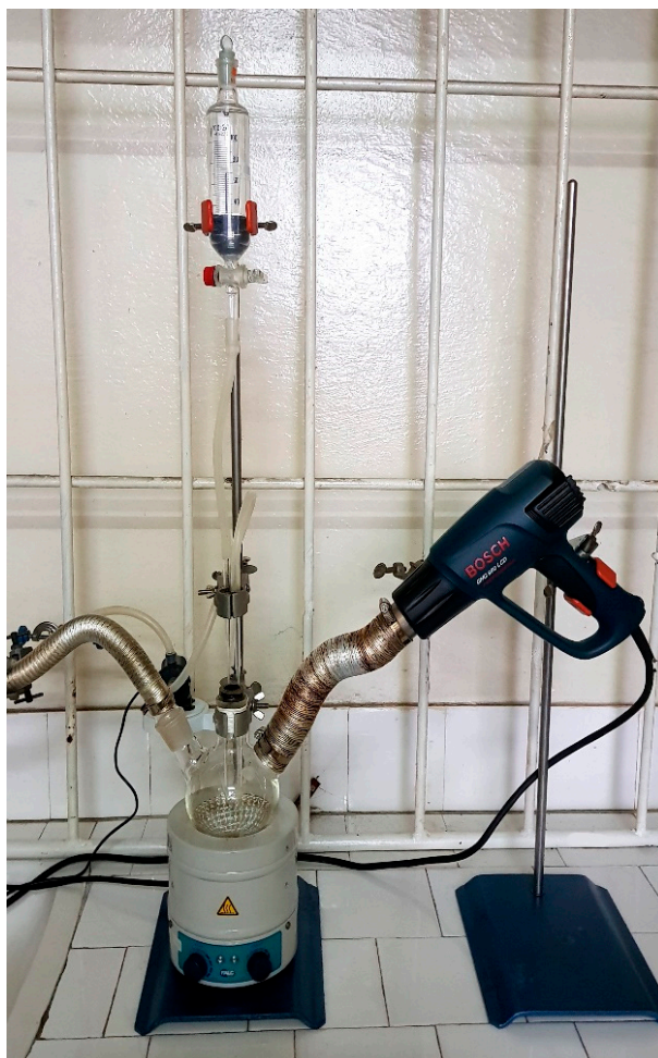
Figure S1. Experimental setup used to prepare carbon dots.
