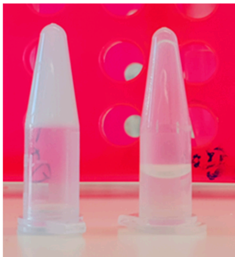
Figure S9. Crosslinking of oxidized inulin with ADD resulting in the formation of inulin hydrogel.
