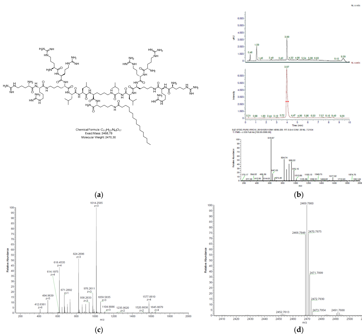
Figure S7. (a) Structure of G2 RR-Palmitamide (RR)4(KLL)2KKC16, it was obtained after manual synthesis as foamy colorless solid after preparative RP-HPLC (7 mg, 3.5%). (b) Analytical RP-HPLC: t_r = 3.99 min (100% A to 100% D in 7.5 min, \lambda = 214 nm). (c), (d) MS (ESI+): C_{112}H_{221}N_{45}O_{17} calc./obs. 2468.78/2468.78
