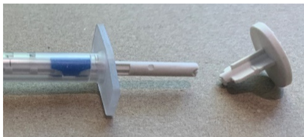
Figure 4. Picture of a broken plunger tops. (A) Participant used excessive force while pressing the plunger rod. (B) Broken when the participant exerted a lateral force of the plunger rod, snapping off the top of it.
