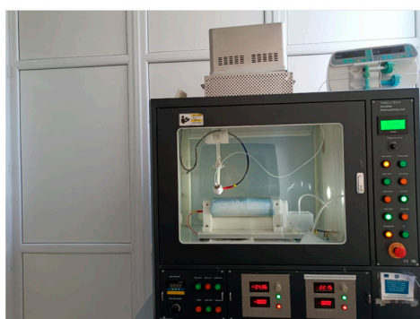
Figure S3. Electrospinnig of fish scale gelatin dispersions on polypropylene sheet.
