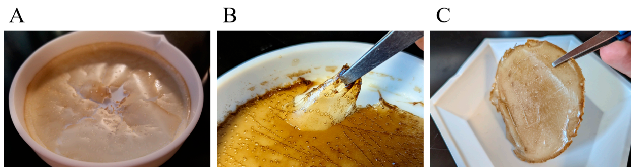
Figure 1. Various EPS films (A) EPS film without crosslinker and antibiotic. (B) EPS film with the addition of EDC. (C) EPS film containing EDC crosslinker and amikacin antibiotic. The amikacin film displays a malleable, uniform, and robust texture.
