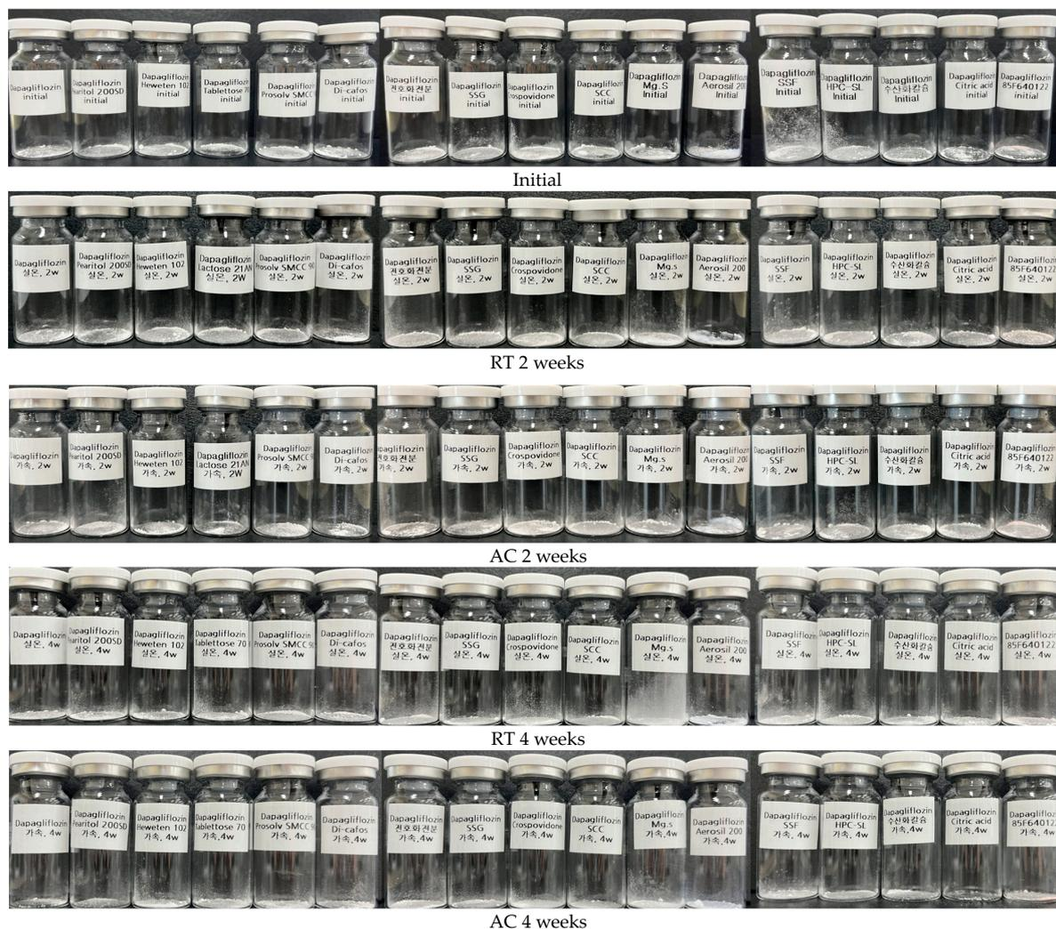
**Figure 7.** Appearance of compatibility test between dapagliflozin propanediol hydrate and various excipients; RT, room temperature storage condition; AC, accelerated storage condition.
