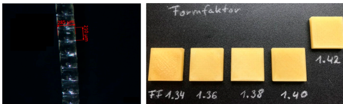
Figure 3. (Left): Strand produced with HME pellets containing PVA 4-88 and 10% KTZ; (Right): Determination of FF using five cubes with different FF (20 mm \times 20 mm \times 4 mm).
