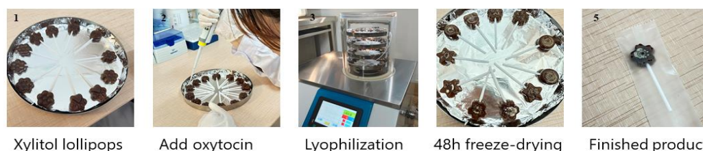
Figure 3. Method (left to right) for producing sugar-free (xylitol) lollipop candies with oxytocin acetate (OXT) freeze-dried on one surface of the lollipop (‘oxipops’).
