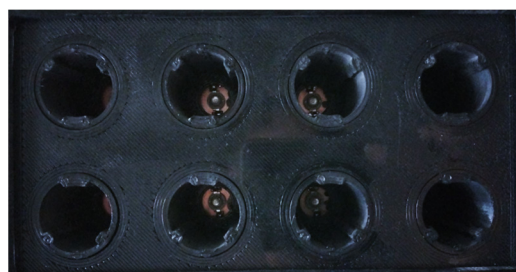
Figure 4. LED array for eight test tubes using a 3D printing lab rack grid.
