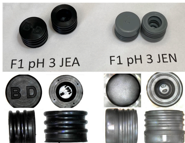
Figure 3. Visual (up) and micrograph (down) aspect of the two different tested sealing gaskets (JEA left and JEN right) located in the glass syringes of formulation 1 pH 3 of the autoinjectors after 53 months of storage at 25 \pm 2 °C.
