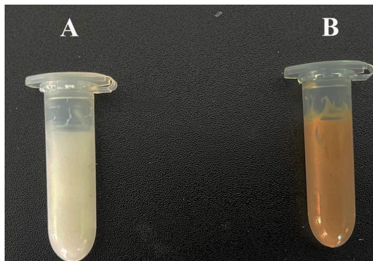
Figure 1. Photograph of cream base (A) and PTC (B) formulations after the centrifugation test.
