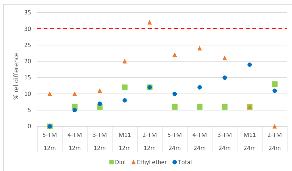
Figure 4. Comparability between different temperature models with the parameter of relative difference, where 5-TM represents the 5-temperature model (FM), 4-TM represents the average of 4-temperature models (M1–M4), 3-TM represents the average of 3-temperature models (M5–M10), and 2-TM represents the 2-temperature model (M12). The red line represents the relative difference limit of 30%.
