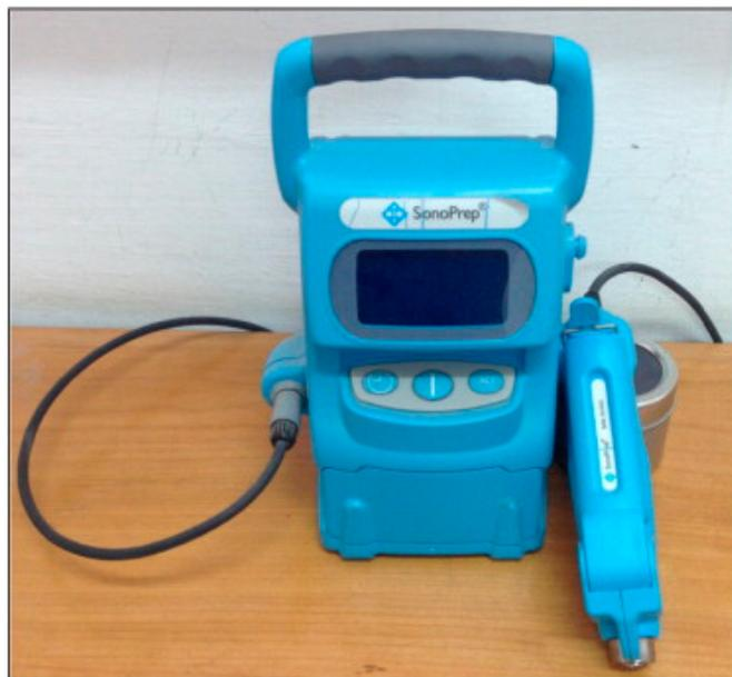
**Figure 7.** The SonoPrep<sup>®</sup> ultrasound device (Reprinted from [50] with permission. Copyright 2014 Elsevier).
