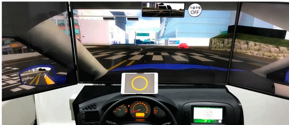
Figure 2. Experimental Environment with Simulator and Intelligent Driving Assistant.
