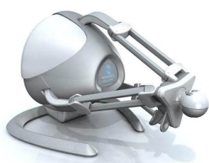
Figure 4. Novint Falcon haptic device used in interactive visuo-haptic environments.
