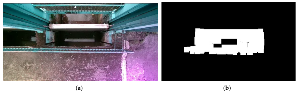
Figure 2. (a) Captured frame from camera experiencing chromatic aberration in bottom right of the scene. (b) Thresholded region which forms the basis for the ROI coordinates.
