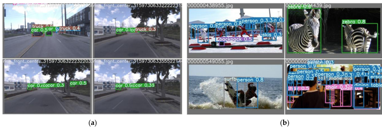
Figure 10. Test results of the proposed NextDet's sparse and dense object detection along with confidence scores on the validation set of images. Image (a) provides object detection result on the Argoverse-HD dataset, and image (b) provides object detection result on the COCO dataset.
