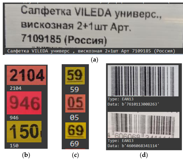
Figure 12. (a) Description segment recognition; (b) Rub segment recognition; (c) Kop segment recognition; (d) Barcode decoding using pyzbar library.
