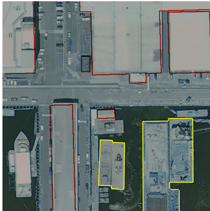
Figure 12. Aerial image with marked building footprints from cadaster (red) and moored vessels (yellow).
