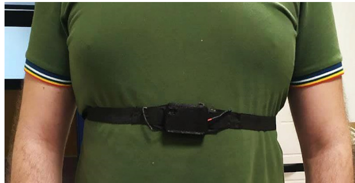
Figure 8. Breathing rate sensor worn on the user's chest.
