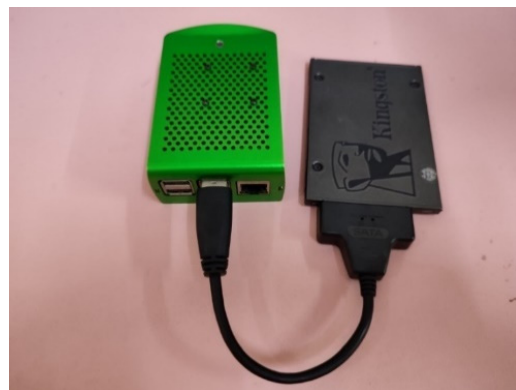
Figure 5. External SSD connected to a Pi 4B.
