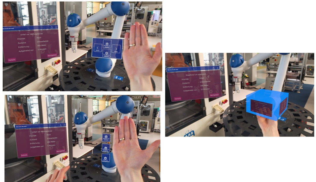
Figure 6. View of the three variations for our hand menu evaluation. Upper left: click menu; lower left: scroll menu; right: cube menu.
