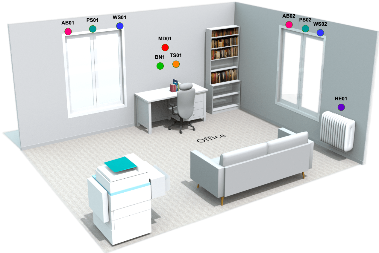
Figure 17. Overview of the sensors and actuators in the smart office scenario.
