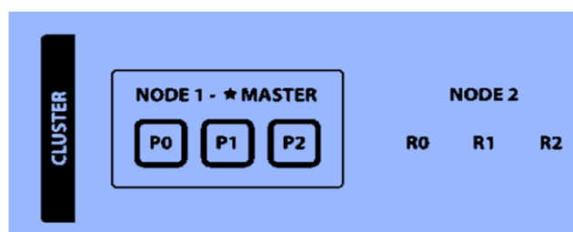
Figure 2. Example with 2 nodes, 3 primary shards each with a replica shard.
