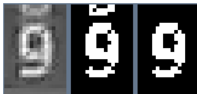
Figure 7. Initial image taken using camera on edge device, intermediate image after B/W conversion and the final image without artifacts.
