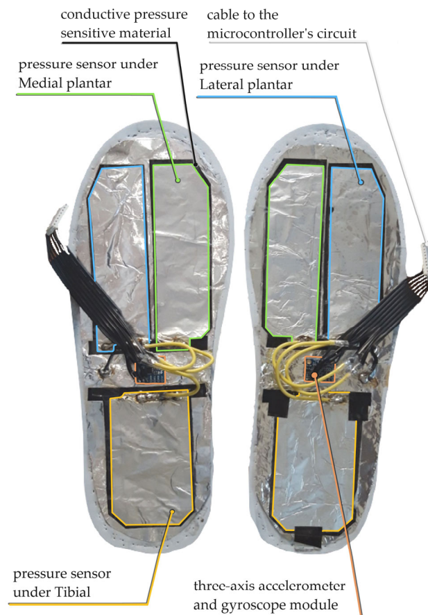
Figure 2. Experimental insoles with installed sensors.
