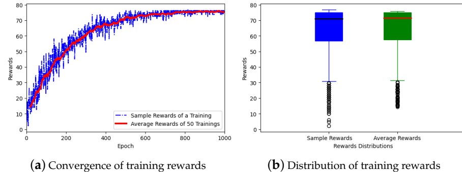
Figure 17. Visualization of training a DRL model: The total rewards over 1000 epochs demonstrate consistent improvement, with performance approaching a near-optimal policy after 700 epochs, where the rewards stabilize around 75, as shown in line graph (a). The box plot (b) reveals that the majority of training epochs achieve an average reward of 70, which represents the median value.
