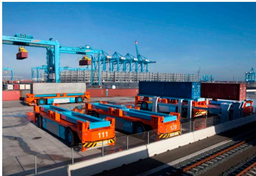
Figure 6. Electric automated guided vehicles (AGVs) at APM Terminal. Reproduced with permission from [15].
