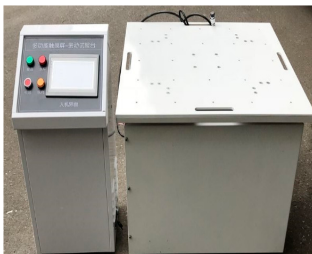
Figure 8. ZD/AB-XTP Vibration Test Bench.
