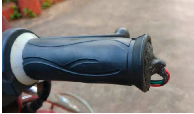
Figure 3. Throttle integration using a potentiometer.
